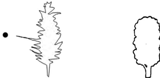
Figure 3: Vegetation Shapes Tested for Horizontal Conductor-to-Vegetation Gaps – Branch Protruding Toward Conductor and Columnar
