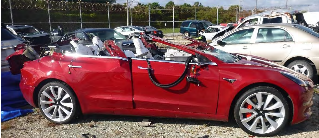
Figure 18. The 2018 Ouchi after striking the side of a semitrailer in Delray Beach, Florida.
